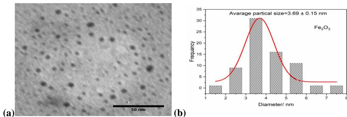
**Fig. 1.** Characterization of Fe<sub>2</sub>O<sub>3</sub> -NPs. (a): (TEM) micrograph and (b): (F) frequency size distribution by TEM.
