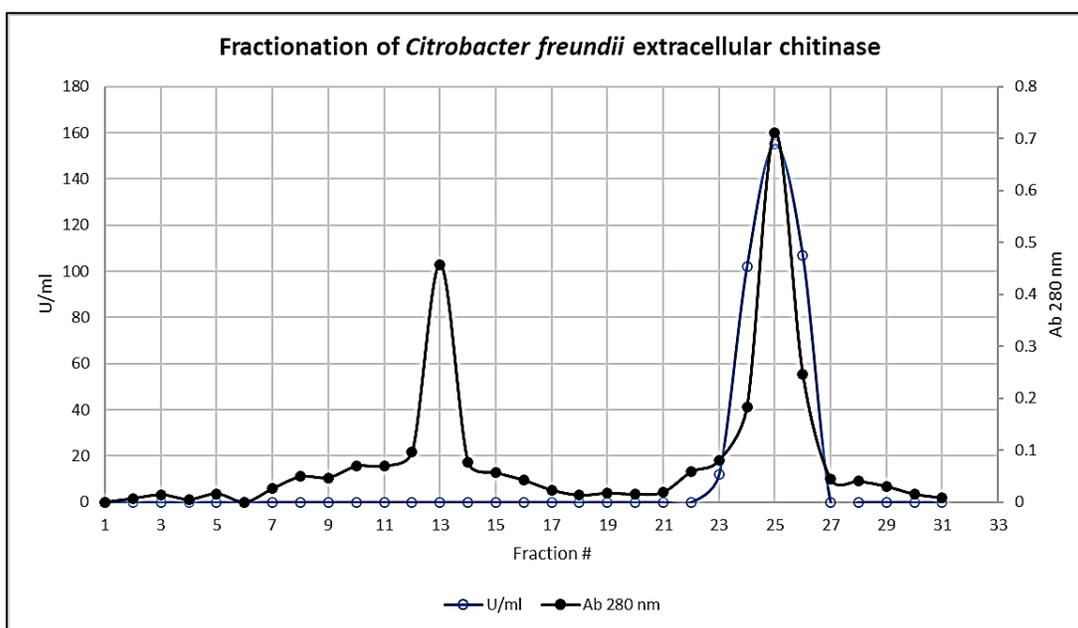
**Fig. 4.** Fractionation pattern of *Citrobacter freundii* extracellular chitinase. After dialysis, purified enzyme was applied to Sephadex G-100 column.
